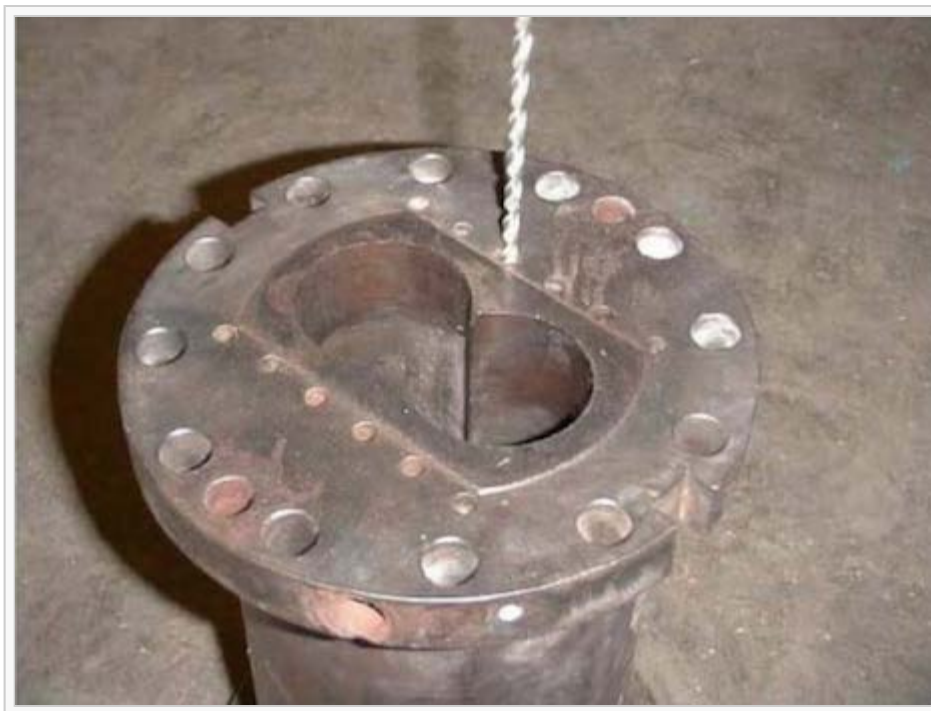
Figure 1: Twin screw barrel having clogged bores drilled out
