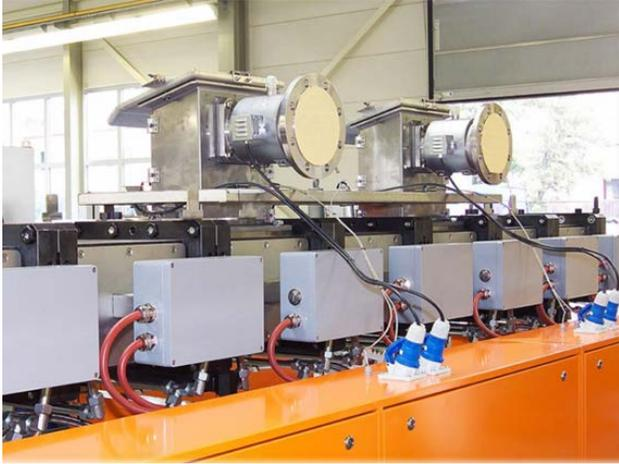
**Figure 9: Heated vent stack**
