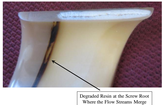
Figure 15. Photograph of a segment from a Maddock solidification experiment for a PVDC resin extrusion. The dark band is degraded resin due to a long residence time at the location.
