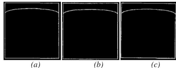
Fig. 3 Interface shape predicted by a purely viscous simulation. The distance from the square entrance is (a)  $0$ , (b)  $0.42 L$ , and (c)  $2.42 L$ , with  $L$  being the length of the side of the square [3].
