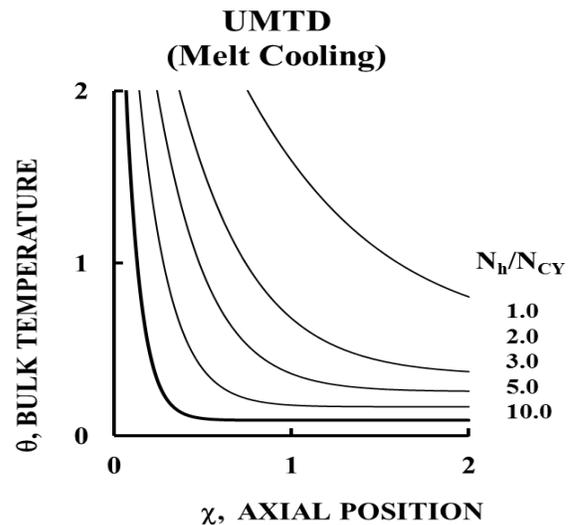
Figure 4. Melt Cooling The temperature of the melt entering the melt zone is greater value than the prevailing fully developed melt temperature.
