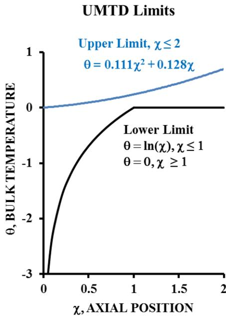
Figure 3. Upper and Lower Limits of Melt Temperature Heating
