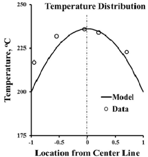
Figure 6. Temperature Distribution for LDPE Model based on UMTD analysis of bulk temperature distribution.
