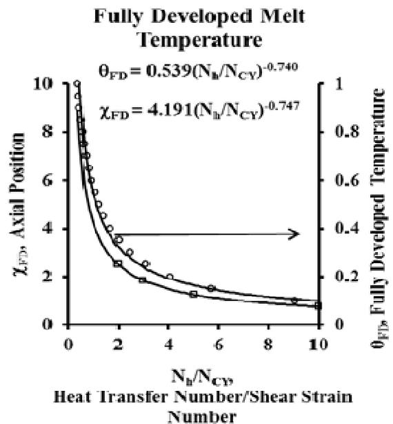
Figure 2. Axial Position Number at which Fully Developed Melt Temperature Begins and Fully Developed Temperature. They are a function of only heat transfer and shear strain numbers.
