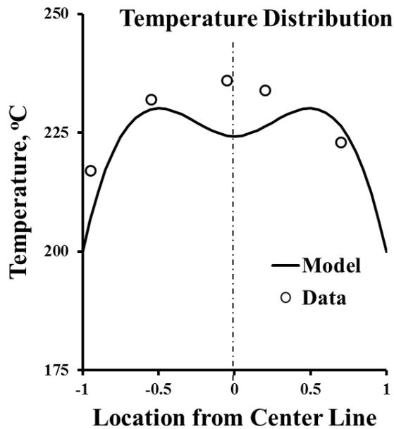
Figure 7. An “M” Shaped Profile The average product temperature for the model is the same as for the data.
