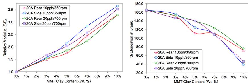
Figure 3. Tensile properties for constant Q/N samples run on a ZSK-18mm extruder with MMT fed in the rear or side ports.
