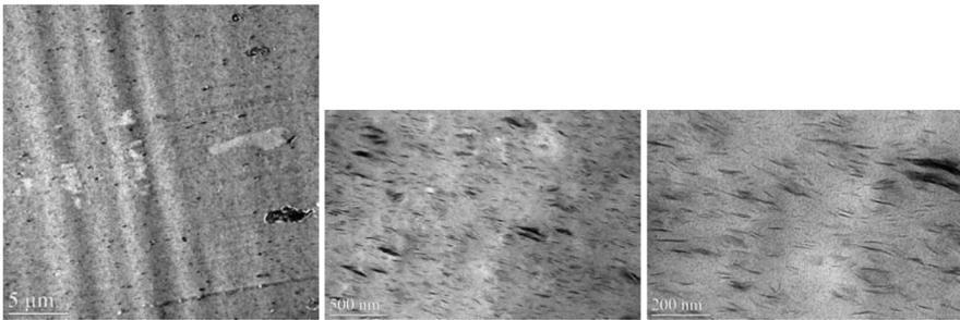
Figure 14. Zinc ionomer / organically modified Laponite OG composites (5 wt. % clay) TEM.
