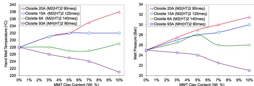
Figure 4. Sodium ionomer / organically modified MMT extrusion melt temperature and pressure.
