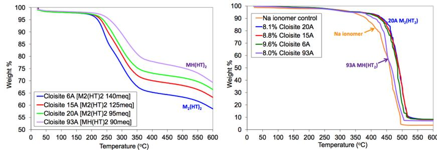
Figure 15. Thermogravimetric analysis (TGA) of organically modified MMT and sodium ionomer nanocomposites in air.
