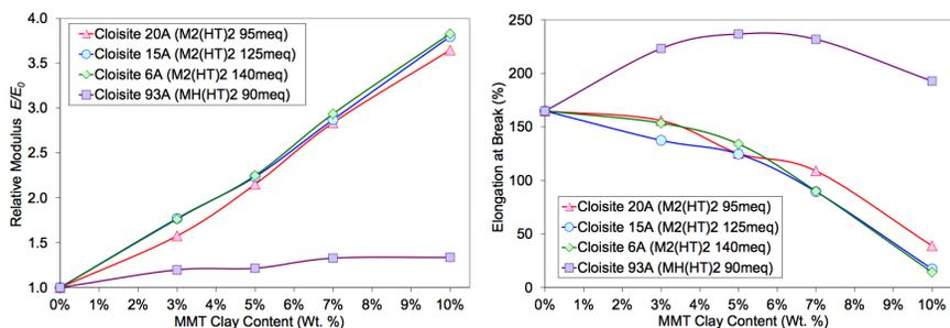
Figure 5. Sodium ionomer / organically modified MMT tensile properties.
