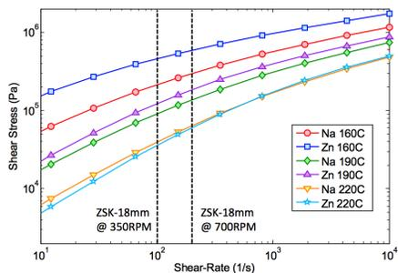
Figure 1. Sodium and zinc ionomer shear stress vs. shear rate curves at different operating temperature regimes.
