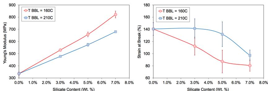
Figure 2. Tensile properties of injection molded bars of letdown extrusions of Sodium ionomer / Cloisite 20A master-batches made under low and high temperature conditions (error bars are  $\pm$  one standard deviation, 6 bars per state).
