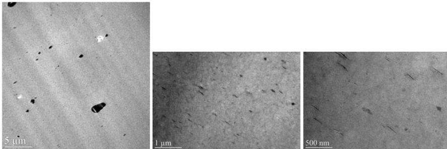
Figure 13. Zinc ionomer / organically modified Laponite B Fluorohectorite composite (5 wt. % clay) TEM.
