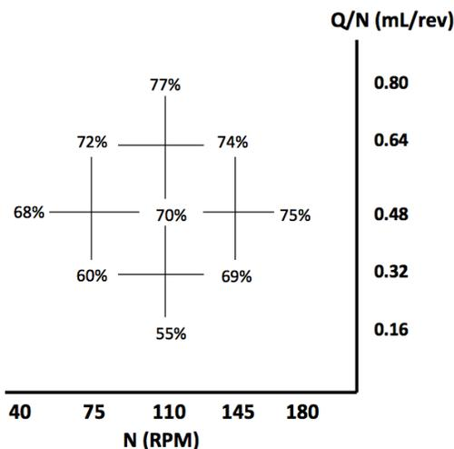
Figure 7. Percent breakup of 92 kPa beads using narrow kneading blocks
