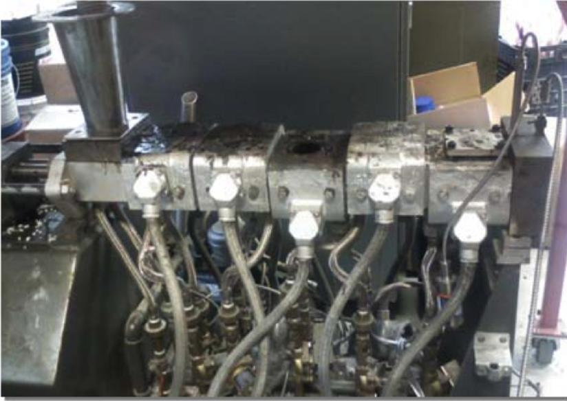
Figure 1. 28-mm Coperion Co-Rotating TSE
