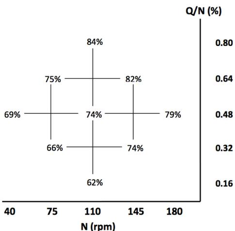
Figure 6. Percent breakup of 92 kPa beads using wide kneading blocks
