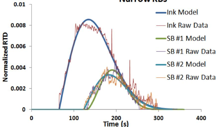
Figure 8. Normalized narrow kneading blocks RTD and RSD curves for .315mL/75rpm condition
