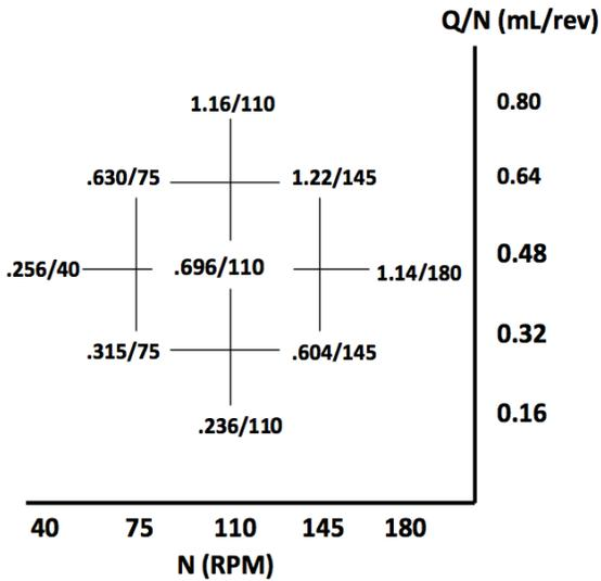
Figure 2. CCD grid of experimental conditions
