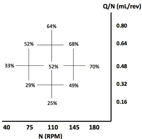
Figure 5. Percent breakup of 119 kPa beads using narrow kneading blocks
