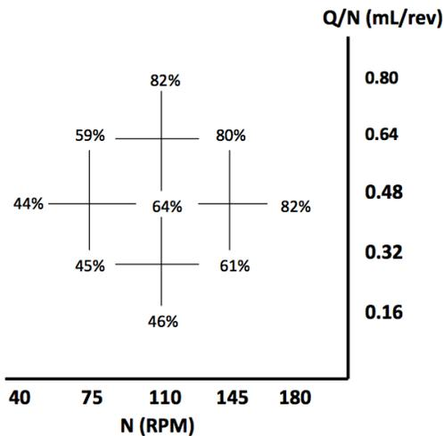
Figure 4. Percent breakup of 119 kPa beads using wide kneading blocks
