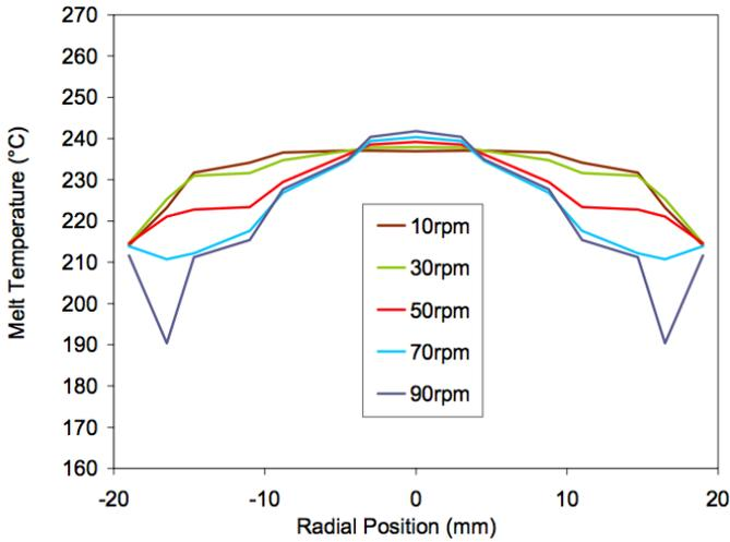
Figure 9 Melt temperature homogeneity; effect of screw geometry and screw rotation speed
