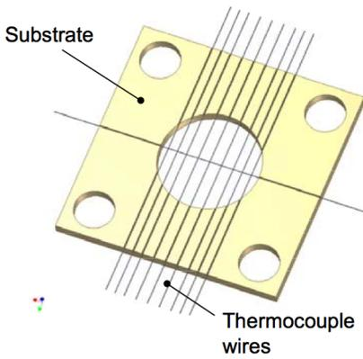
Figure 2 Thermocouple mesh sensor
