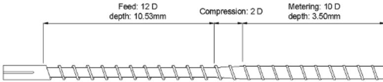
(b) Single flighted, 3:1 compression ratio, with rapid or stepped compression
