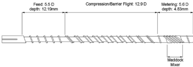
Figure 3 Extruder screw geometries
