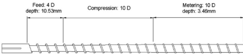
(a) Single flighted, 3:1 compression ratio, with gradual or tapered compression
