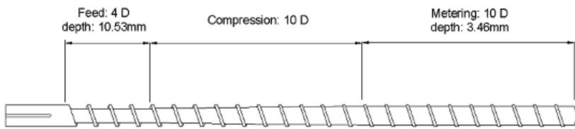
(a) Single flighted, 3:1 compression ratio, with gradual or tapered compression
