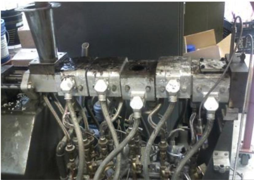
Figure 1. 28-mm Coperion Co-Rotating TSE
