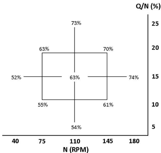
Figure 4. Percent breakup using wide kneading blocks
