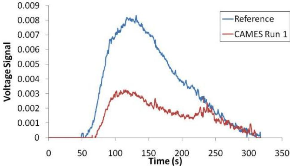
Figure 6. Normalized wide kneading blocks RTD and RSD curves for .236/110 condition
