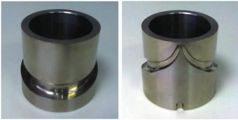
Figure 8. Photographs showing the front (left) and back (right) geometries of a crosshead style die.
