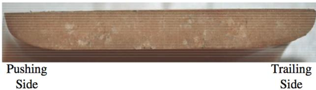
Figure 2. Photograph of a specialty powder resin that is melting via the one dimensional melting mechanism. Even at this early location in the melting process, the thickness of the melt film adjacent to the barrel wall was thicker than normal.
