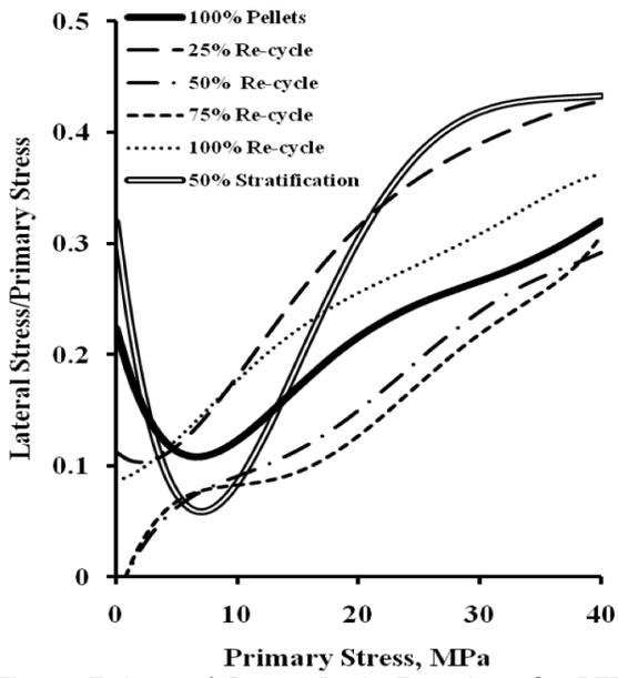
Figure 7. Lateral Stress Ratio Functions for PET/Re-cycle Mixtures
