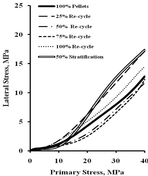
Figure 6. Regression Functions for Lateral Stress versus Primary Stress A 6th order polynomial is used for each set of
