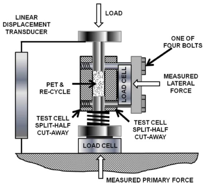
Figure 2. The Test Cell for Measuring the Primary and Lateral Forces During Compression of Bulk Resin Feed as a function of bulk density [1,2]. Diameter of the cylinder is 12.7 mm. The linear displacement transducer records the height of the sample to establish the evolving bulk density value and lateral area of force.
