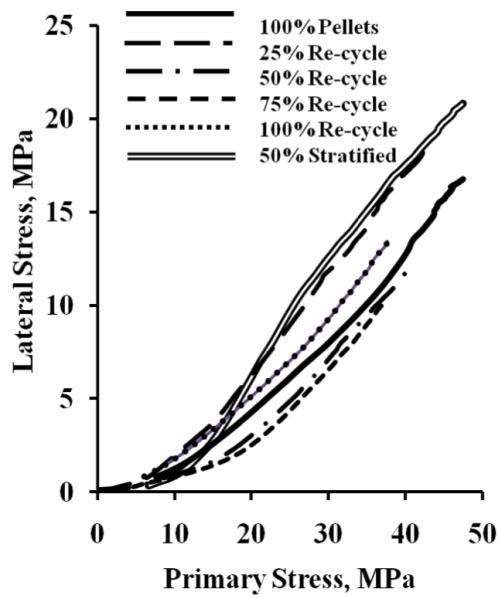
Figure 5. Raw Data for Lateral Stress for PET Pellets with Re-cycle vs. Primary Stress
