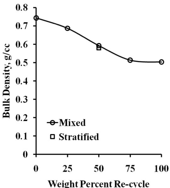
Figure 3. Bulk Density of PET Feed versus percent of Re-cycle Flakes. Values are those measured with the test cell before load is applied.
