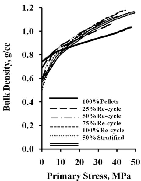
Figure 4. Data for Bulk Density of the Pellet/Re-cycle Mixtures vs. Primary Stress
