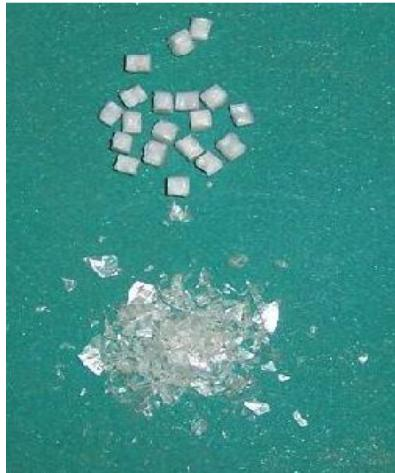
Figure 1. PET Resins. Bottom is re-cycle scrap and the top is virgin PET pellet. Different mixture ratios of these two components were tested. Pellet dimensions are about 3.2 x 4.2 mm.
