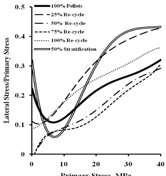
Figure 7. Lateral Stress Ratio Functions for PET/Re-cycle Mixtures
