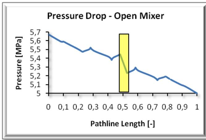
Figure 5. Pressure profile through the open fluted mixer
