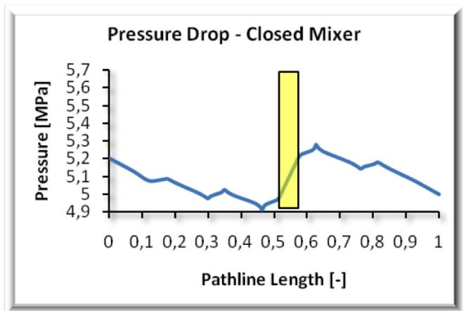
Figure 6. Pressure profile through the closed fluted mixer
