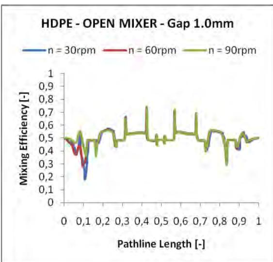
Figure 9. HDPE Mixing efficiency of the open fluted mixing element
