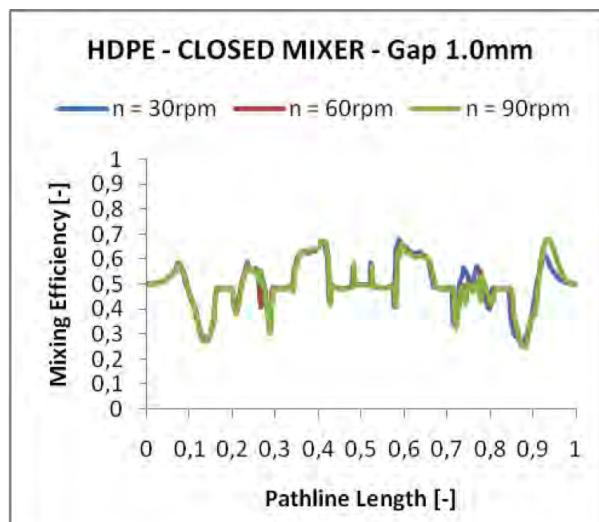
Figure 11. HDPE Mixing efficiency of the closed fluted mixing element
