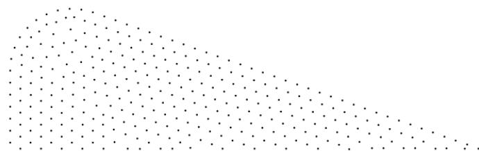
Figure 5. Node distribution for the RFM modelling of secondary flows in a teardrop shape duct.
