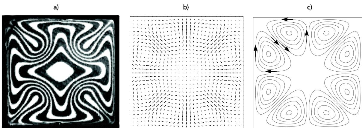
Figure 2. Polystyrene Secondary flows in a square channel: a)Experimental Results. b) RFM prediction. c)FEM prediction
