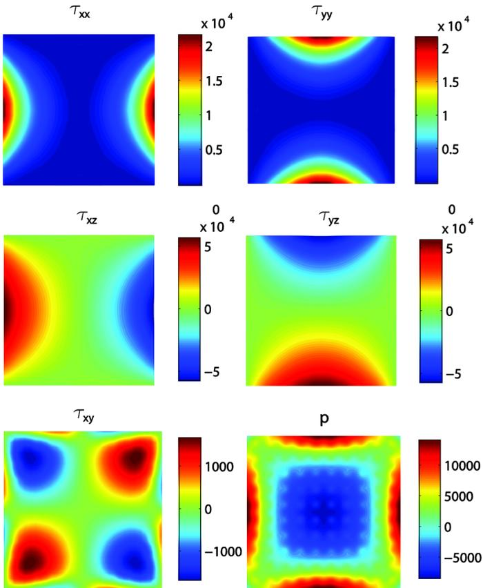
Figure 4: Stress tensor components and pressure values (Pa) for a square duct flow prediction
