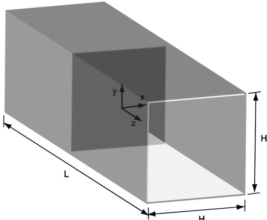
Figure 1: Schematic diagram of a square duct
