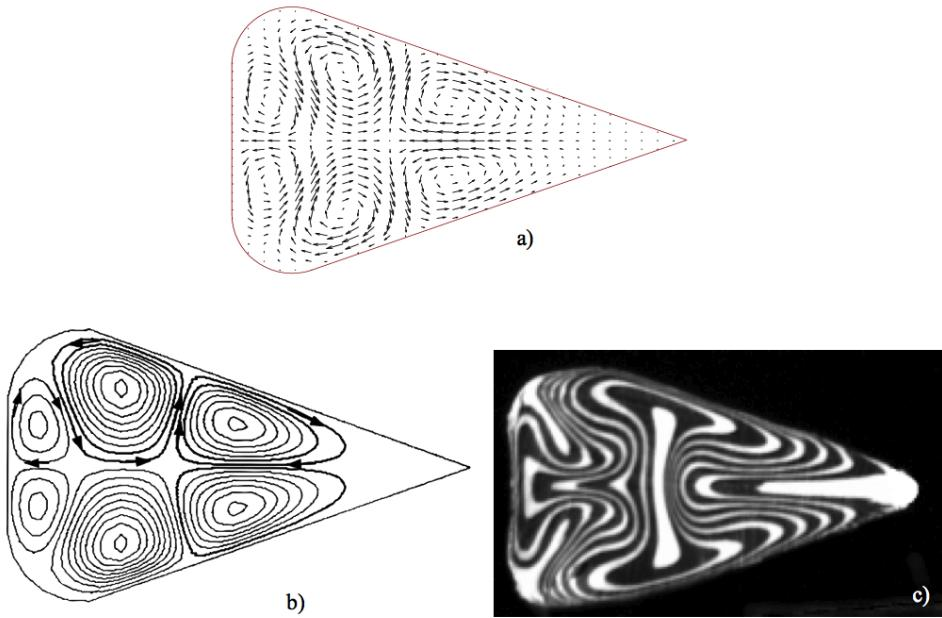
Figure 6. Polystyrene Secondary flows in a teardrop shape channel: a) RFM prediction. b) Dooley's FEM prediction
