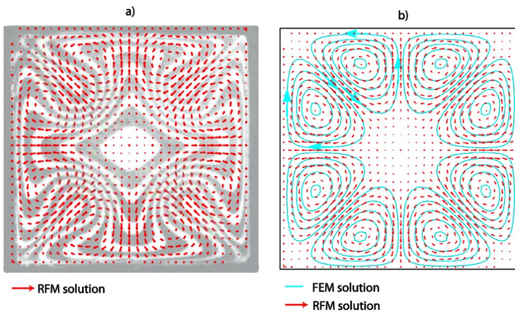
Figure 3: Comparison of the prediction of secondary flows in a square channel of RFM with: a) Experimental Results. b) FEM results
