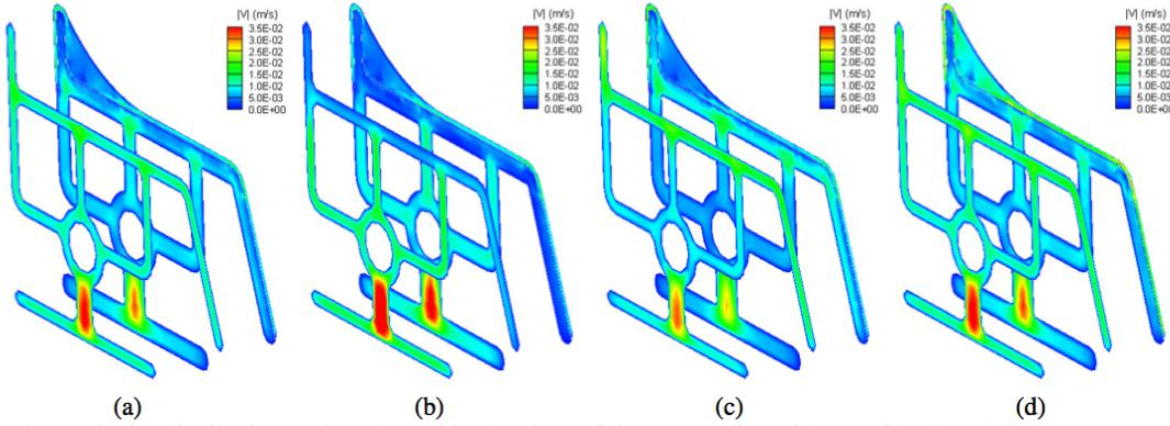
Fig. 9 Velocity distribution at the exit, and in the plane of the contact line of the profile die. (a) Substrate: LDPE-A, Cap: LDPE-A, (b) Substrate: LDPE-A, Cap: LDPE-D, (c) Substrate: LDPE-D, Cap: LDPE-A, (d) Substrate: LDPE-A, Cap: LDPE-A with larger flow rate (LFR) through the cap layer.
