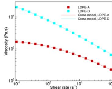
Fig. 2 Viscosity of two different grades of LDPEs [6].
